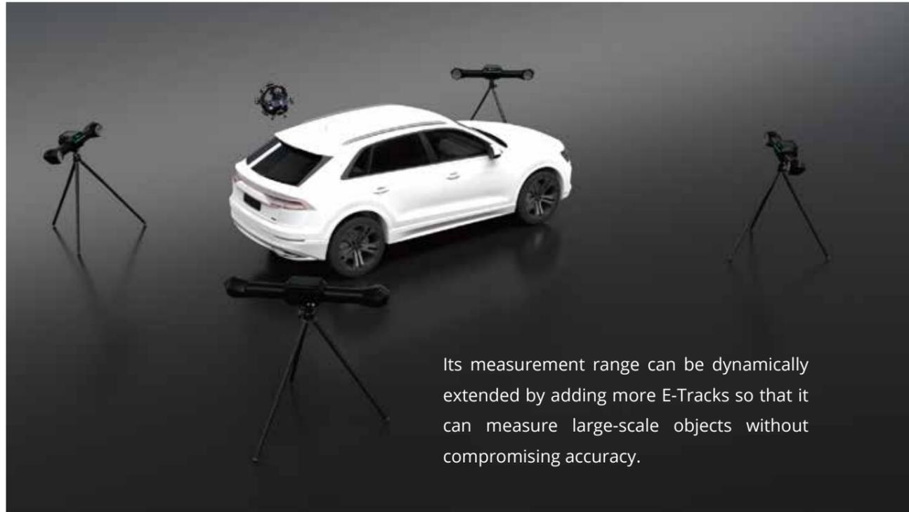
Its measurement range can be dynamically extended by adding more E-Tracks so that it can measure large-scale objects without compromising accuracy.
